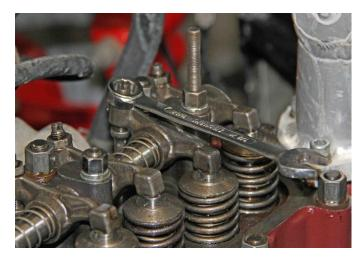
In itself, the described procedure is simple, but age has a way making the simple a struggle when it involves arthritic hands, eyes that have seen better days, a front pulley dog nut on which a tab locking washer interferes with the spanner fit all while observing when the identified valve rocker has reached its maximum opening - the 'tipping point'.
